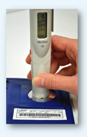
To verify the accuracy of Type 2 gages, the thickness of a series of coated reference standards covering the expected range of coating thickness is measured (*Figure 28, left*) using either the single point of two-point verification process, described earlier for the Type 1 gage. However, in
