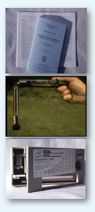
well as the relative humidity, are all within the coating manufacturers' specified range or as required by the project specification. These values (air temperature, relative humidity, surface temperature and dew point temperature) can be obtained using sling (Figure 2, top left) or battery-powered psychrometers (Figure 3, middle left) in conjunction with US Weather Bureau **Psychrometric Tables**
