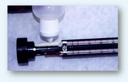
Step 2 -Saturate the wick with distilled water, or fill the water reservoir at the end of the sling
