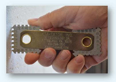
*Immediately* after the wet coating film is applied, insert measuring face into the wet coating, perpendicular to the surface (*Figure* 21, *left*). The two
