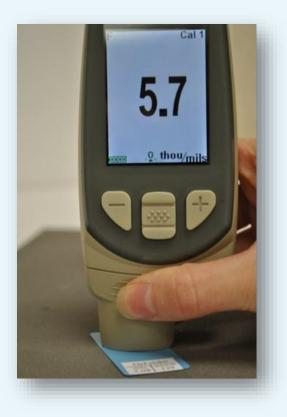
The final step in verifying gage accuracy is to align the Type 2 gage to a known value to improve gage accuracy on the specific type and design of surface or within a specific measurement range. Some refer to this step as gage optimization. In this case, the gage is adjusted (when
