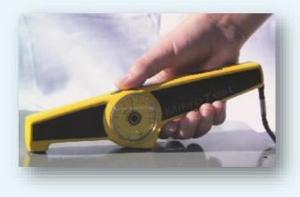
For the Type 1 magnetic pull-off gages (*Figure 24, left*), a permanent magnet is brought into direct contact with the coated surface. The
