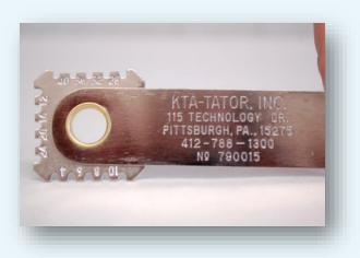
All notch-type gages contain four or eight faces with a series of steps, with notches between the steps. Each step is numbered. The number corresponds to the wet film thickness in mils (0.001") or micrometers (µm). There are 25.4 µm in 1 mil.
