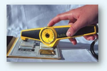
To verify the accuracy of Type 1 gages, the thickness of a series of coated reference standards covering the expected range of
