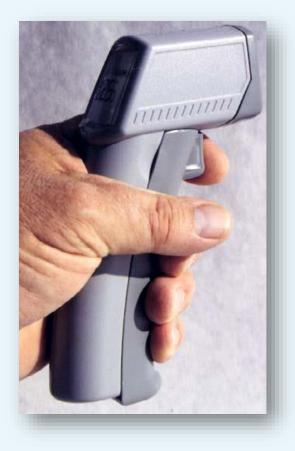
Non-contact infrared pyrometers (*Figure 16*, *left*) can also be used to measure surface temperature. These gages are often equipped with laser sightings, so that the user can target the location on the surface to be measured. However, the further away from the surface that the "gun" is held, the larger the area of
