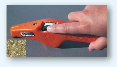
Once the Type 1 thickness gage is verified for accuracy, the next step is to measure and record the Base Metal Reading
