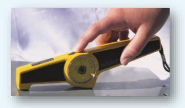
There are two common types of coating thickness gages including Type 1 (magnetic pull-off) (top left) and Type 2
