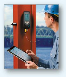
The measurement of air temperature, relative humidity, dew point temperature, and surface temperature is oftentimes required before and during coating application activities (*Figure 1, right*). Air or surface
