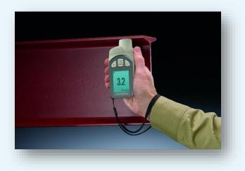
Type 2 electronic gages use electromagnetic principles and electronic circuitry to convert a reference signal and display it as
