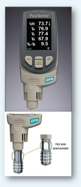
As an alternative to sling and battery-operated psychrometers, digital psychrometers can be used to determine the prevailing weather conditions (Figure 13, top left). These gages digitally display the air temperature, relative humidity, dew point temperature and surface temperature essentially at the push of a button. One manufacturer features a hot wire probe to monitor wind speed (Figure 14, bottom left). Although the
