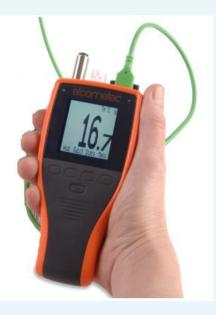
Ambient conditions should be measured and recorded prior to mixing the coating materials and at 4-hour intervals thereafter, unless conditions appear to be declining. In this case, more frequent checks may be required. The prevailing ambient conditions at the actual location of the work should be assessed. The location, date, time of day and the conditions of air temperature, relative humidity, dew point temperature, and surface temperature should be recorded.
