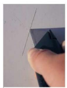
Starting at the intersection of the "X," the tip of the knife blade is used to attempt to lift the coating from the substrate or the underlying coating layers (Figure 32).
