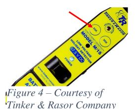
(see Figure 4) that are used to indicate the sensitivity of the device. For the model shown, the detector should signal and the LED should light when the 80K (80 ohm) button is pressed, provided the detector is to be used on coated steel structures and it is in calibration. The 90K (90 ohm) setting is for coatings on concrete.
